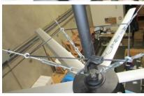
THE CORD IS CUT TO A PREDETERMINED LENGTH FOR PROPER TENSION. DO NOT EXCESSIVELY STRETCH THE CORD.
