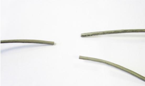
2. Strip jacketing off the three CAT5 cables and separate each color wire leaving approximately 2 inches of each wire exposed including the drain/shield wire.
